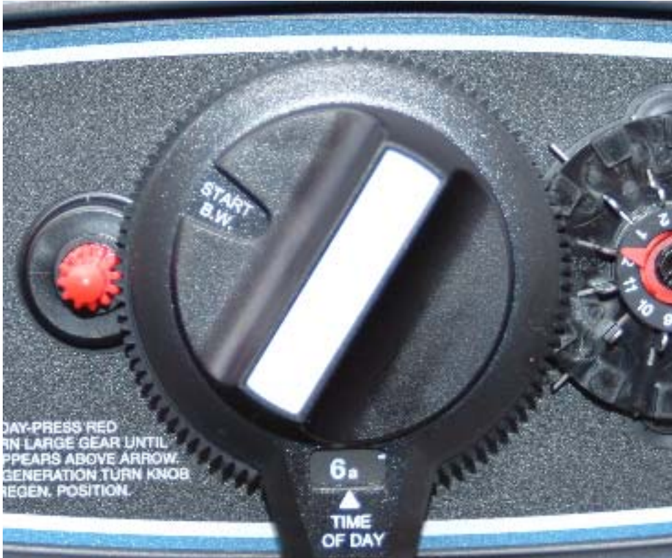
Filter entering the Backwash (B.W.) mode
