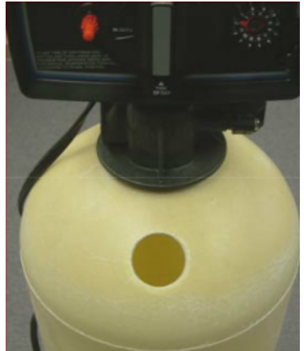
Dome Hole Plug Removed
