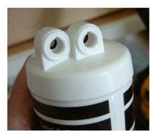
Step 8 Insert the new cartridge, bottom end first.
