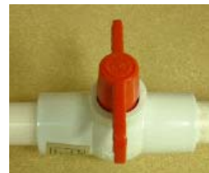
Valve in the 'closed' position.
